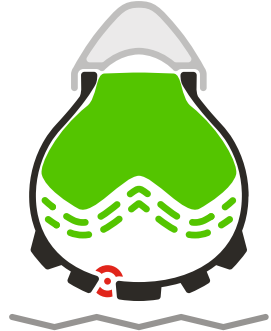
RUN FLAT Foam expansion in case of puncture
